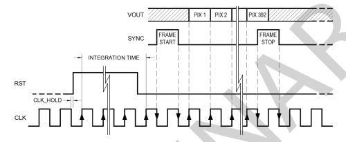
Integration time is set by holding RST high for the desired number of clock cycles. Exposure starts when HIGH on RST is sampled on the rising edge of CLK, and ends when LOW on RST is sampled on the rising edge of CLK. For example, a 10ms integration time can be achieved with a 50kHz CLK by holding RST high for 500 clock cycles.
